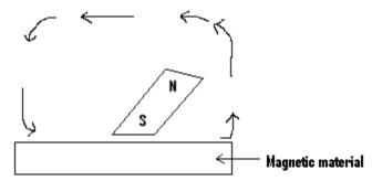
(i) In this method, the magnetic material to be converted into the magnet is placed on a table.
